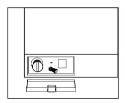
After draining out the water through the drain plug, open the coin trap by rotating in anti-clockwise direction and remove the foreign particles like coins, pins, hooks, present if any. Tighten the coin trap and drain plug to their original positions and close the bottom door.
