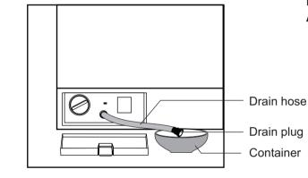
Place a shallow container near the bottom door. Pull out the drain hose and open the drain plug to drain out the water from the machine in the container.
