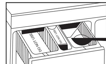
Normal-wash chamber: (Marked-I), to be filled with - detergent during every wash programme. Do not fill detergent in other chambers.
