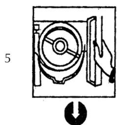
Replace filter and screw on tightly to avoid leakage of water
