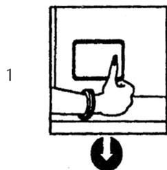
Open door flap by pressing on the right hand. Clean filter under running water
