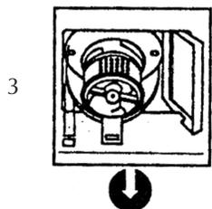
Turn Fluff Filter cover anti-clockwise drain water into container and take out filter
