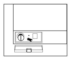
After draining out the water through the drain plug, open the coin trap by rotating in anti-clockwise direction and remove the foreign particles like coins, pins, hooks, present if any. Tighten the coin trap and drain plug to their original positions and close the bottom door. 4 BEFORE USING THE MACHINE AGAIN, RUN THE MACHINE WITH-OUT CLOTHES AND DETERGENT BY SELECTING ANY SHORT WASH PROGRAMME. THIS WILL ENSURE THAT THE WATER SYSTEM LINE GETS FILLED WITH WATER.
