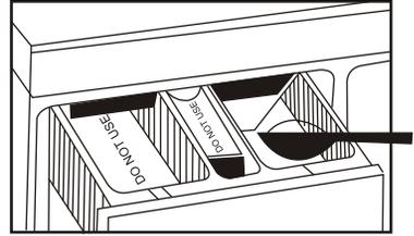
Normal-wash chamber: (Marked-I), to be filled with - detergent during every wash programme. Do not fill detergent in other chambers.
