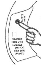
The dryer is equipped with a temperature activated safety cut out device. The safety reset button is near the door latch and is used to reset the safety device.
