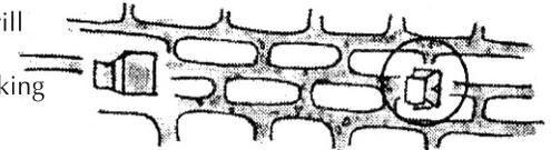
**Note:** When fixing the brackets to the wall, the mounting plate should be facing toward the other bracket.
